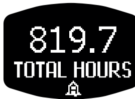
Figure 1-13: Quick View Main Screen with Alarm "Bell" Icon
