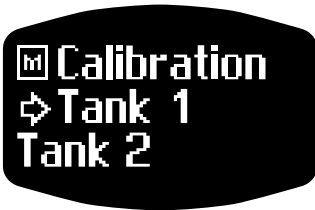
Figure 1-49: Selecting a Fuel Tank to Configure.
